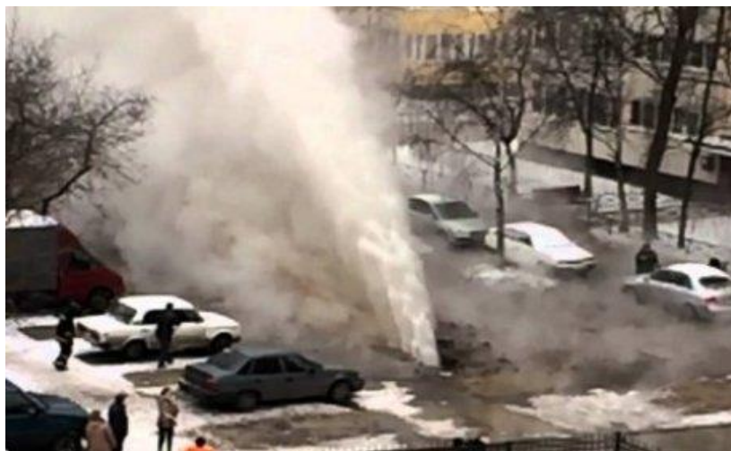
Figure 2. Pipeline explosion in Almaty city
